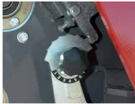
SIMPLE AND ACCURATE BALE DENSITY ADJUSTMENT
