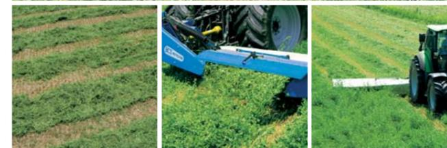
The rear mounted disc mowing machines are at the basis of the **ROTEX design**. Available in four versions, **Rotex Silver 4**, **Rotex Silver 5**, **Rotex Silver 6** and **Rotex TSB 7**, they differ in the dimensions of the cutting equipment and the typology of the load bearing structure.
