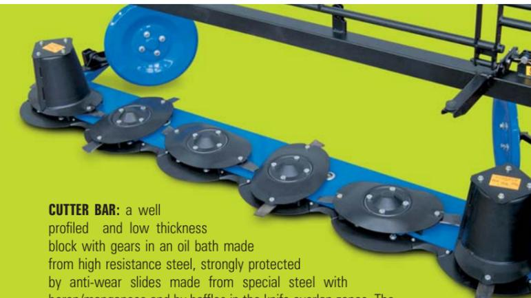
**CUTTER BAR:** a well profiled and low thickness block with gears in an oil bath made from high resistance steel, strongly protected by anti-wear slides made from special steel with boron/manganese and by baffles in the knife overlap zones. The highly aggressive profiled discs are made from special steel. The profile of the bar allows better penetration in all types of forage, even if thick and flattened, making it easier to pass through without clogging.
