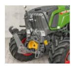
2,540 daN lift capacity is available on the fully integrated front linkage in the P variant. Then there's the vibration damping so you can work in safety and comfort.
