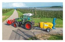
Efficient combination of processes. With the 540E/750 front PTO, you can drive the mulcher at the operating speed, though the sprayer in the rear and the tractor operate at a reduced engine speed.
