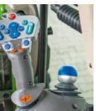
Four double-acting valves on the right-hand and two valves on the left-hand side, together with return flow and cross connection, permit optimal supply of highlevel hydraulic combinations. You can use up to 3 mounts at the same time for time and cost-saving combinations.
