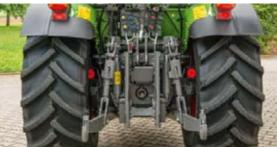
A fully-fledged Cat2 power lift is available in the P-variant. All connections are clearly arranged and easily accessible on all variants.
