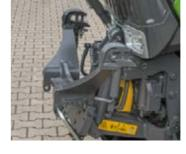
The lower links of the fully integrated front hydraulics can be folded compactly in just a few steps. The compact design makes the 200 Vario particularly manoeuvrable even with a front attachment.
