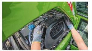
The easily accessible air filter with pre-cleaner delivers maximum performance in air flow and filter life. It is compact and particularly wellsealed. Benefit: low maintenance.
