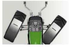
The VarioActive function allows you to achieve full steering lock with just one turn.
