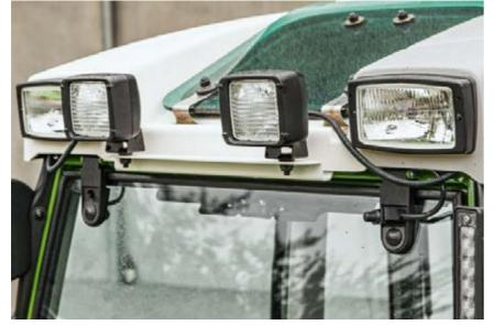
□ Two work lights can also be fitted at the front in the version with auxiliary headlights.
