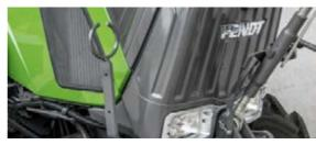
□ The hydraulic hoses are always neat and clutter-free thanks to fasteners at both sides.
